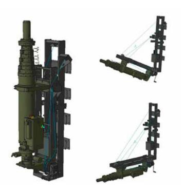
The 90° tilt mechanism is a unique device that is suitable for mounting on the outside of a vehicle or other structures. This mechanism allows for the tilting down of an electromechanical mast to a reachable horizontal position so that important payloads can be mounted easily in place.
